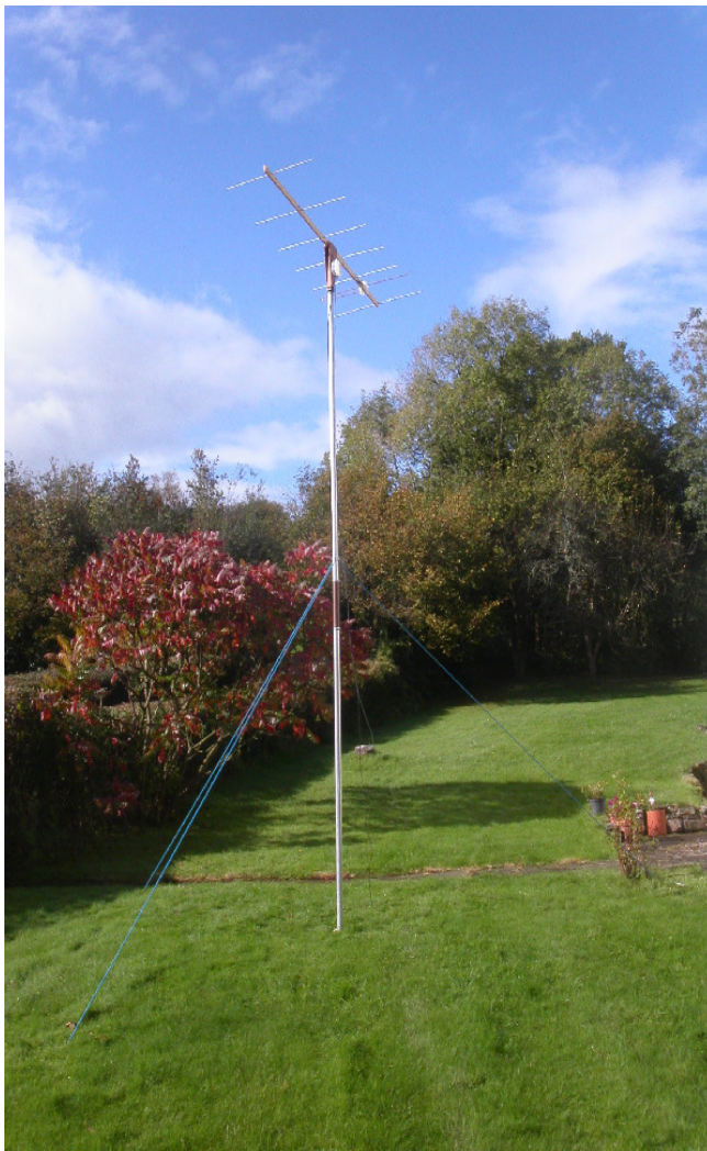
Figure 6.3 7 Element Yagi on a Mast
