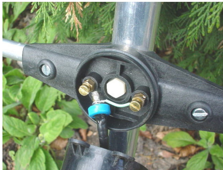
Figure 2.3 Direct connection to dipole feed point
