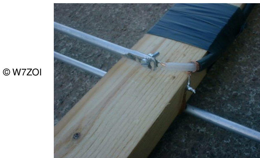
Figure 2.7 Cable connection to driven element
