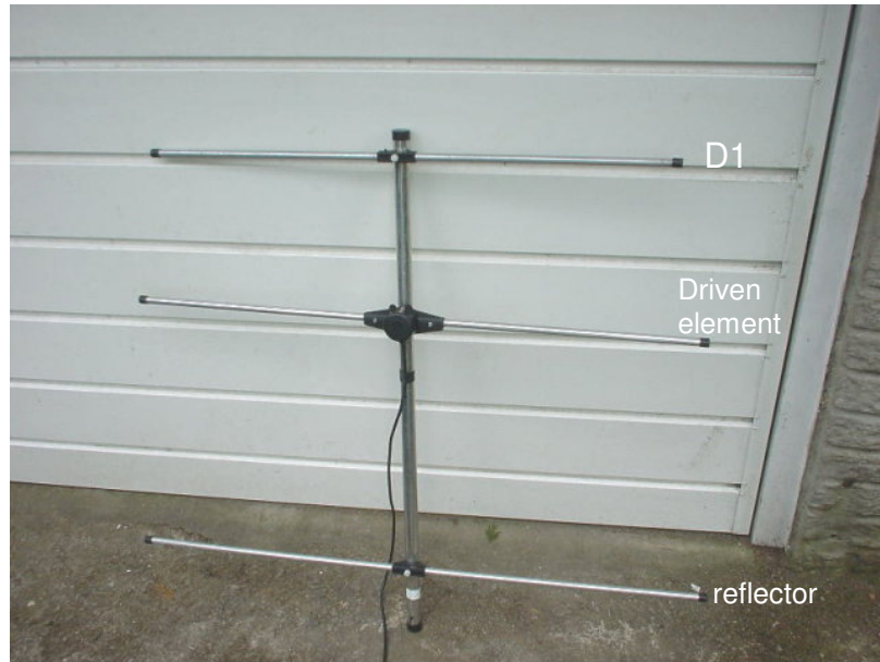
Figure 2.2 A 144MHz 3 element Yagi by G4CQM
