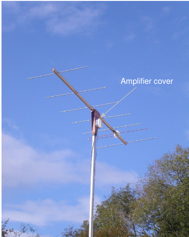
Figure 6.4 7 Element Yagi on mast
