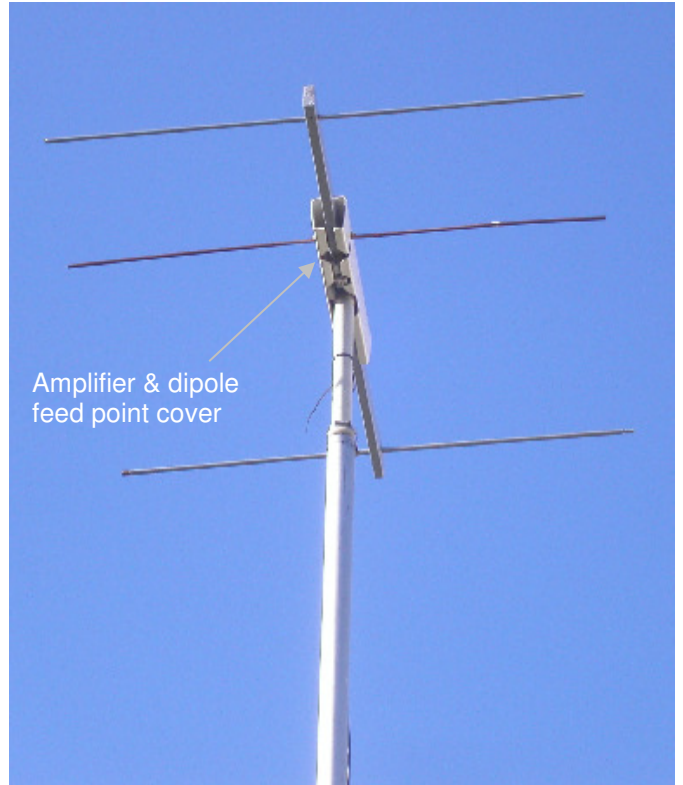
Figure 6.5 3 Element Yagi on mast
